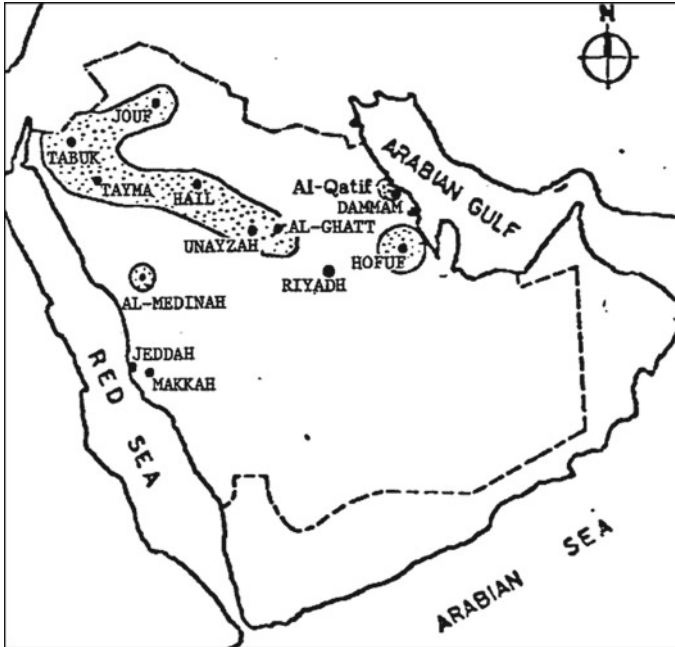
Fig. 11.4 Tentative distribution of expansive formations in Saudi Arabia. Source Dhowian et al. (1985)
