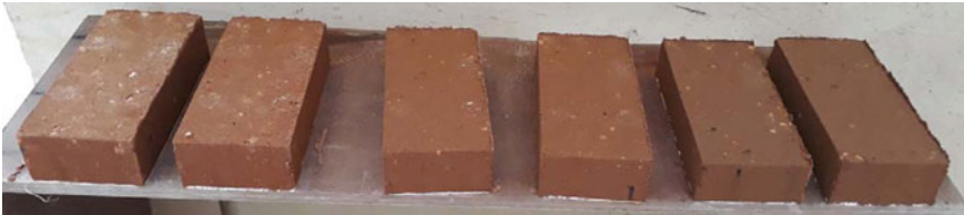
Fig. 11.9 Crack-free fresh compressed stabilised earth block (CSEB) before curing. Source Author, 2017
