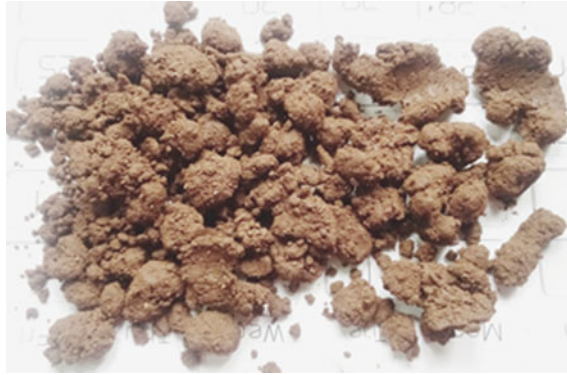
Fig. 1.5 Increase in alkalinity and clay content resulted in the lumpy mix
