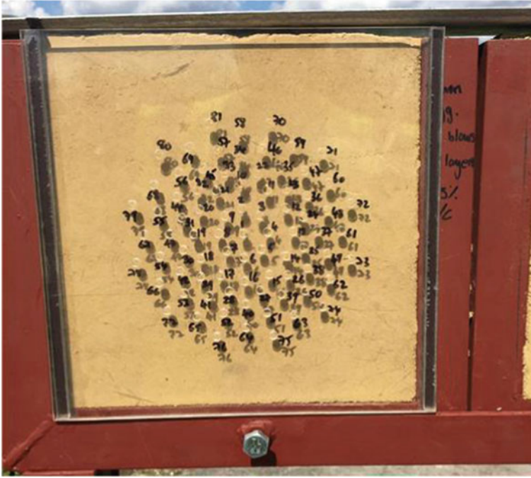
Fig. 28.8 A template fixed firmly onto specimen for measurements
