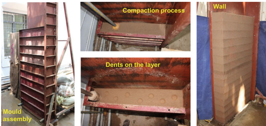
Fig. 26.1 Metal mould assembly, compaction process and CSRE wall specimen
