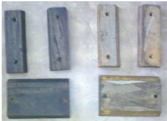
Fig. 14.3 Wooden pieces used in mould for preparing interlocking blocks
