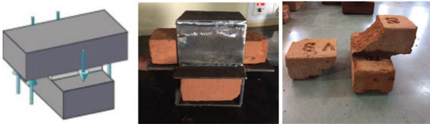
Fig. 19.2 Cross-couplet test tested sample
