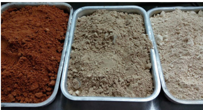
Fig. 11.5 Kharj soil (left), grey marl (middle) and white marl (right). Source Author, 2017
