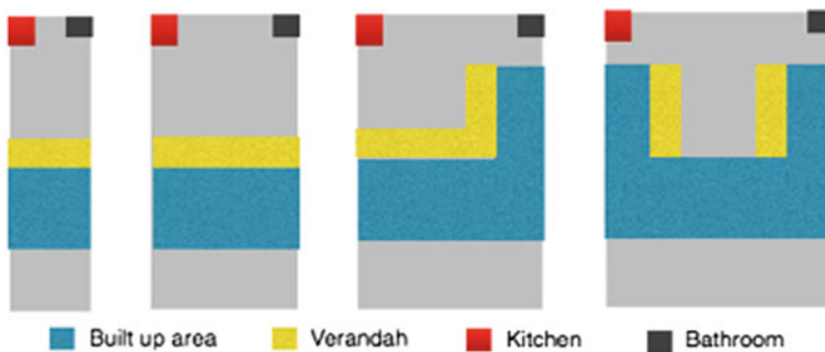
Fig. 36.2 Plan variations of typical Assam-type house
