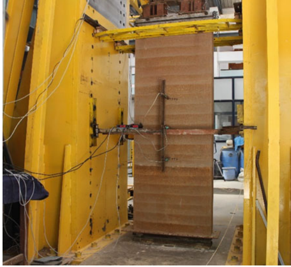
Fig. 26.3 Compression test set-up for CSRE wall
