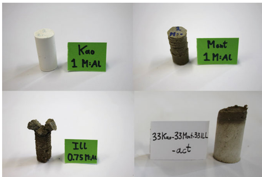
Fig. 2.4 Photographs of activated samples of kaolinite, montmorillonite, illite and a mixture of all three
