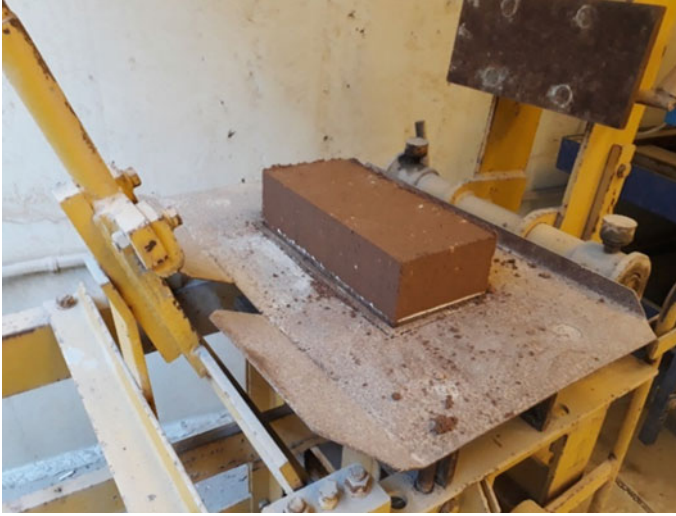
Fig. 11.8 Making earth block in Belgian handpress machine. Source Author, 2017
