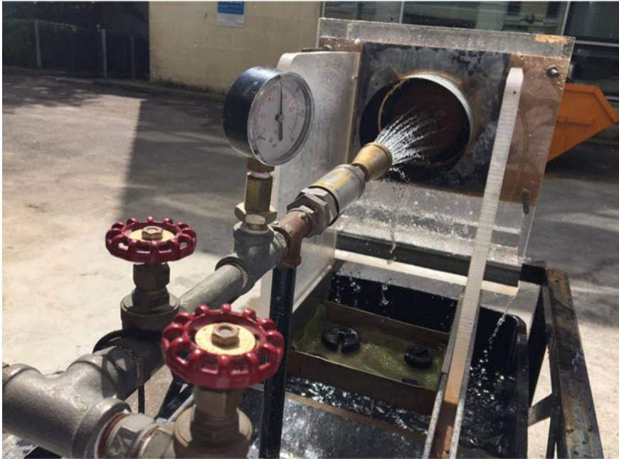
Fig. 28.6 Accelerated spray rig set up and in use
