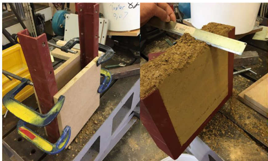
Fig. 28.3 Preparation of rammed earth specimens
