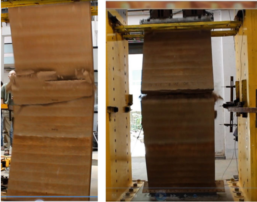
Fig. 26.8 Crushing and flexure tension failures for CSRE walls under eccentric compression
