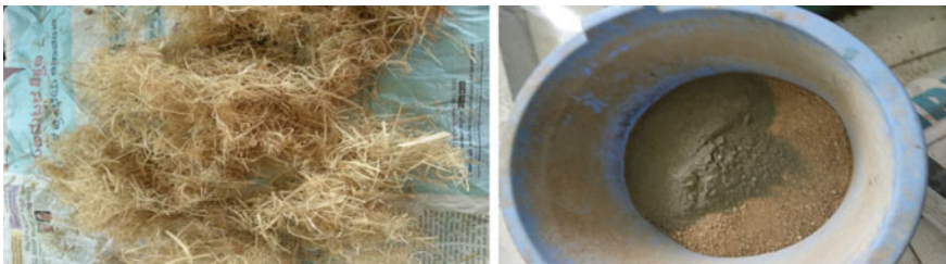
Fig. 21.1 Oven dried bamboo fiber, soil stabilized with cement and C&D
