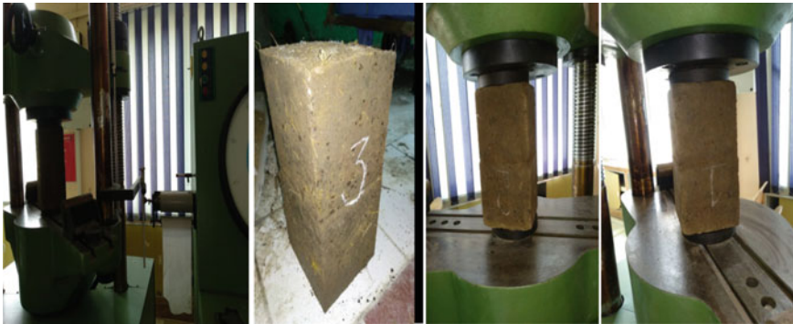
Fig. 21.5 Three specimens under compression
