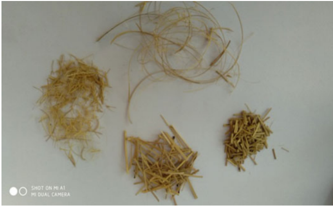
Fig. 21.2 Bamboo fiber diameter 1.156 mm, 2.12 and 700 \mu
