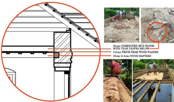
Fig. 37.6 Details of mud roof
