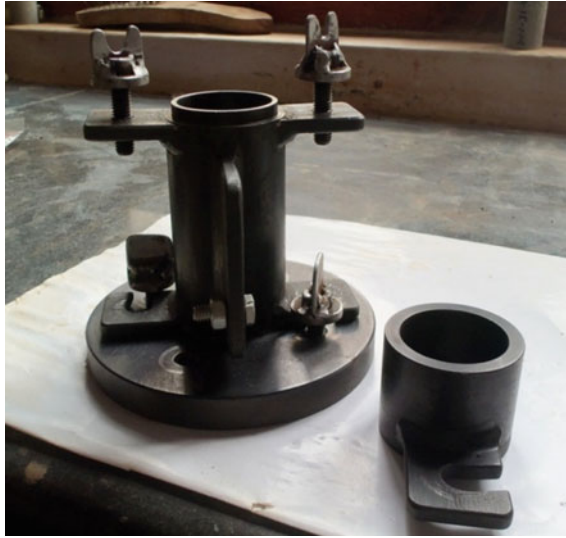
Fig. 5.1 Cylindrical mould used for casting rammed earth cylinders of height 76 mm and diameter 38 mm
