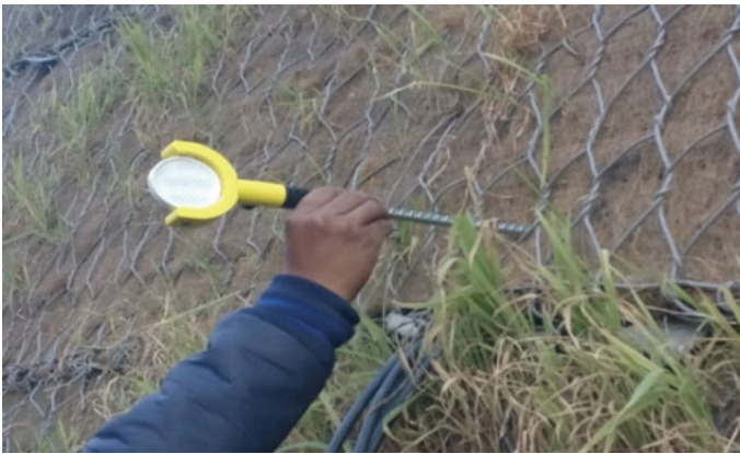
Fig. 19.22 Placement of reflectometer at the site
