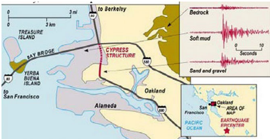
Fig. 11.3 Plan of Oakland area indicating the type of ground, amplification of ground motion at different sites and the location of cypress viaduct that was severely damaged ( https://pubs.usgs.gov/fs/1999/fs151-99/ )
