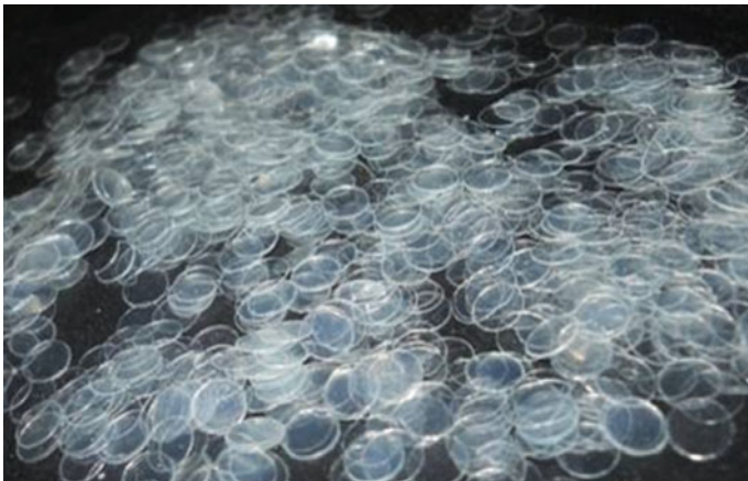
Fig. 3.7 The transparency sheet of 4.5 mm diameter cut for the test
