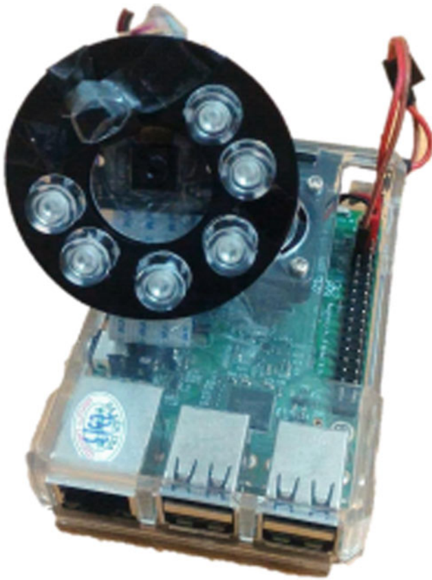
Fig. 5 Hardware design of the image capturing system
