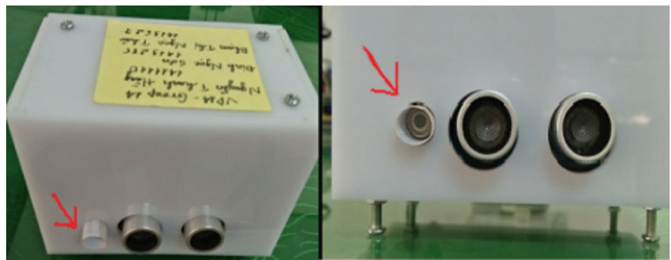
(b) The back side of package with small tube around the IR sensor.
