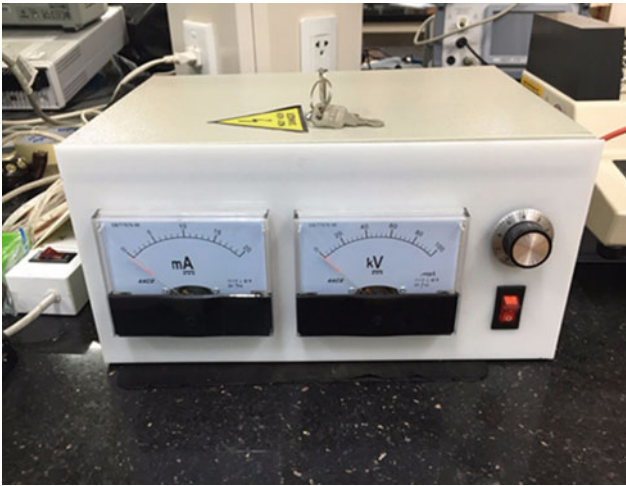
Fig. 10 The high voltage power source after finishing
