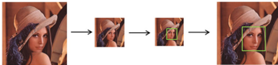
Fig. 4 Shrinking the image then calculate the face rect on the original size image
