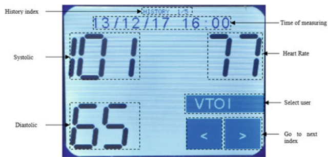
Fig. 3 The LCD with 320 \times 240 in tele-blood pressure
