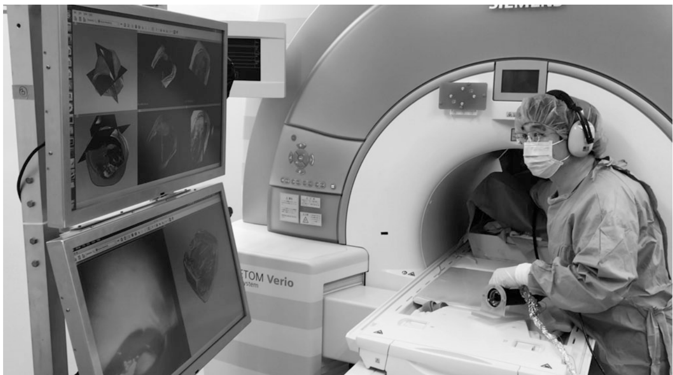
Fig. 3 Experimental setup and trials using the developed MR-compatible endoscope, the navigation software displayed on the MR-compatible in-room monitors, and a 3T MRI scanner
