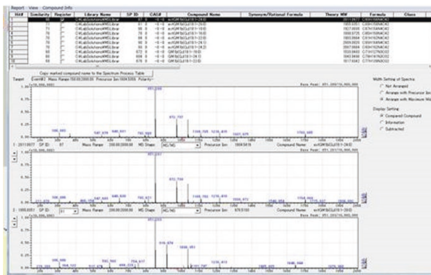
Fig. 1.6 An example of search results of an obtained MS/MS spectrum (top) using the Glycolipid Library distributed by Shimadzu Co., which picks up similar spectra, the middle one having the highest match-score the bottom one the lower score
