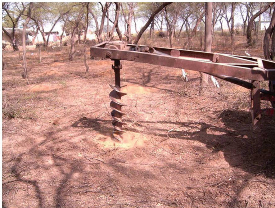
Fig. 4.9 Auger-hole technique used for forestry plantation in a sodic soil
