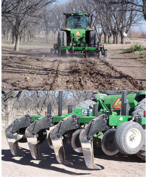
Fig. 9.8 Minimum-till subsoiler. (Photo Courtesy: Texas A&M AgriLife Research Center at El Paso)
