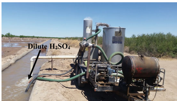
Fig. 9.15 S burner used in a pecan field in the El Paso Valley. (Picture source: Ganjegunte)
