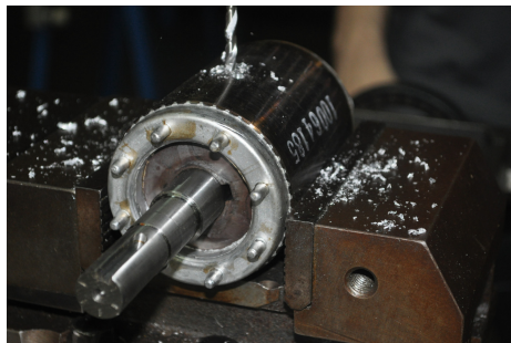
Fig. 3. Artificial generation of broken rotor bars.
