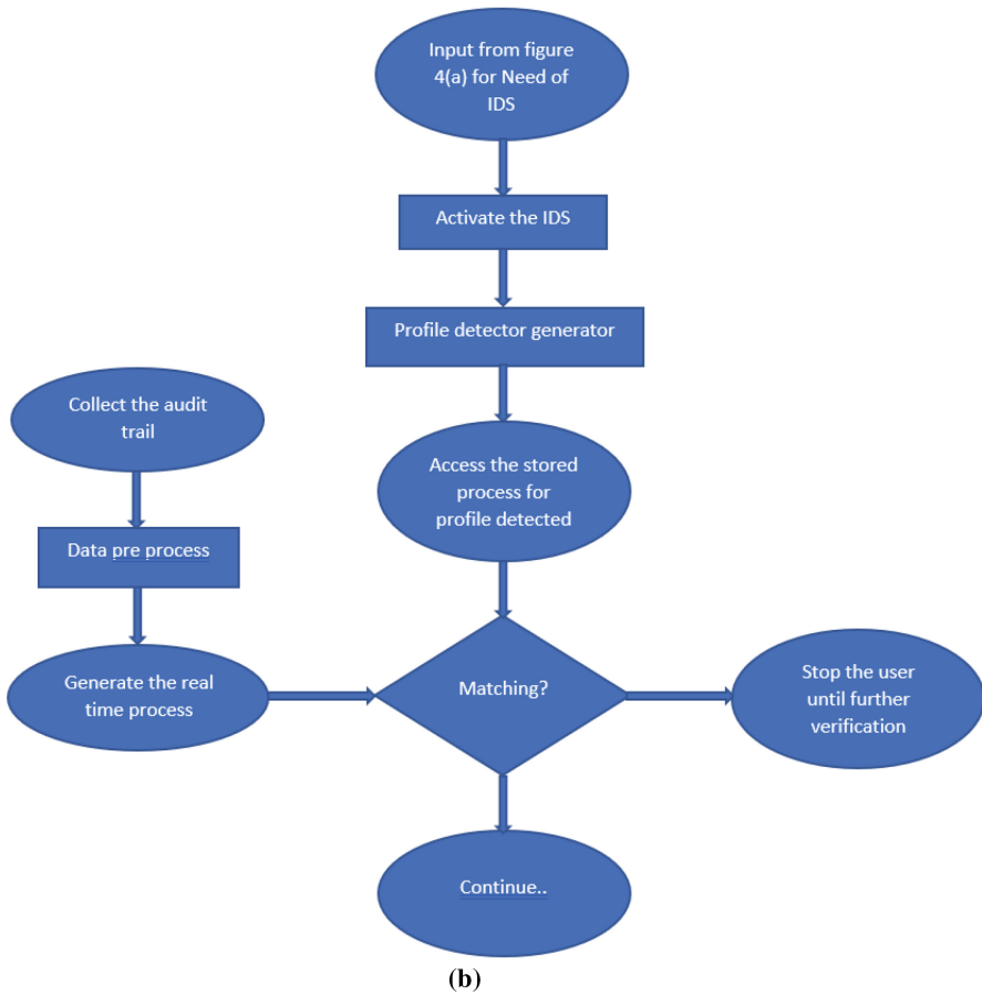
Fig. 5. (a): Process to check the need of Active IDS (b): IDS to detect the suspicious activity in Real-Time
