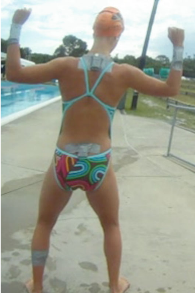
Fig. 4.7 Sensor positions on a swimmer. The sensor positioned at the occipital lobe is hidden by the second swim cap
