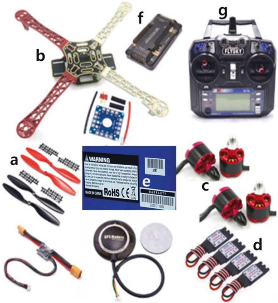
Fig. 3.2 Major drone parts used in assembly procedures a: propeller b: airframe c: motor d: ESC, e: Battery f: FC (flight controller) g: remote controller
