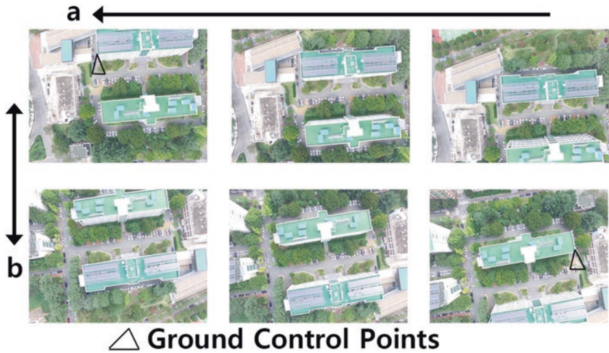
Fig. 6.17 Concept of bundle block adjustment, (a) end-lap (overlap between neighboring images), (b) side-lap (overlap between neighboring strips) Adding another image taken from a different location allows us to intersect the rays and determine the 3D location of the point where the light came from
