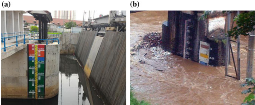
Fig. 2 Water level measuring board a during normal condition and b during high water flow
