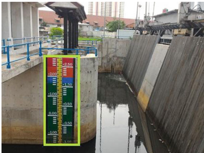
Fig. 7 Detected water level measurement board
