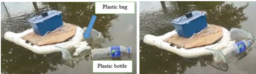
Fig. 5 Waste Hunter surface cleaning
