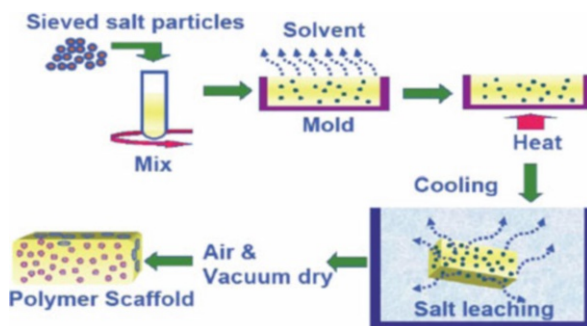
Fig. 27.15 The process diagram of solvent casting technique
