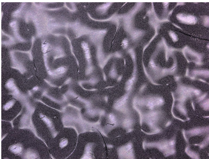
Fig. 1. Surface topography of the pearl photo paper
