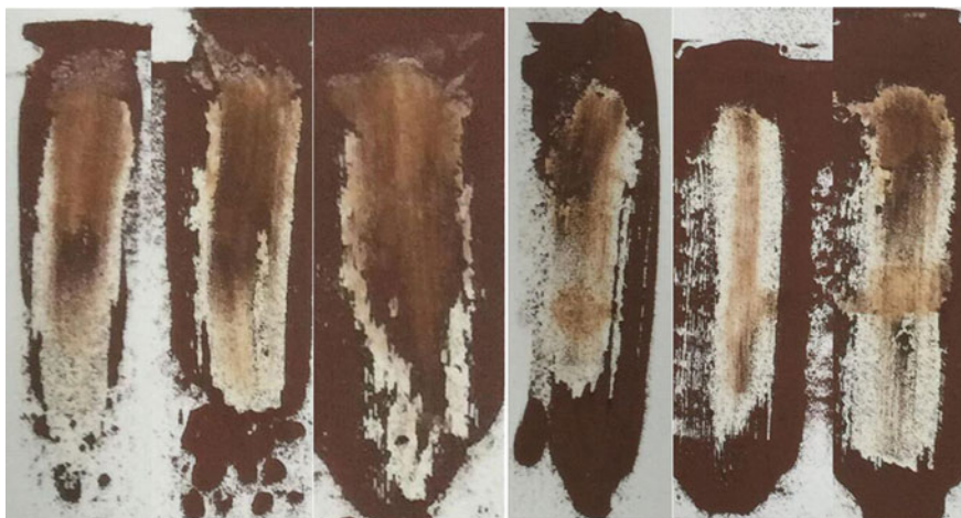
Fig. 4. Drying test of the nanoscale copper ink on the pearl photo paper
