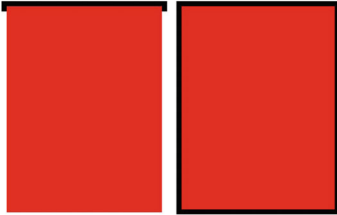
Fig. 3. Effect of not adding the “overflow:hidden/auto;” attribute (left) and the effect of adding the “overflow:hidden/auto;” attribute (right)
