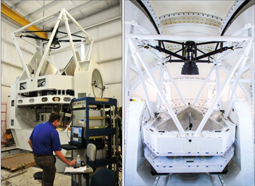
Fig. 26 Two views of the automated 2.4-m Ritchey-Chrétien Thai National Telescope. Left: undergoing testing prior to its installation at the TNO; right: installed and operational at the TNO. (Courtesy: NARIT)
