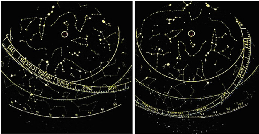
Fig. 3 A comparison of Digital sky star positions (left) with those of the rete of a modern electronic astrolabe (right) with all naked eye stars marked. The astrolabe was made for latitude of 52^\circ , and its star positions are marked by yellow disks. The Digitalsky (Skyskan) stars are white dots
