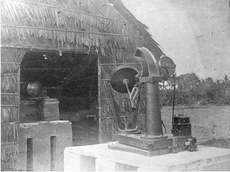
Fig. 18 The siderostat used during the expedition, with its protective cover removed. The associated telescope and spectroscopic camera were located in the adjacent hut. (Courtesy: Royal Astronomical Society)
