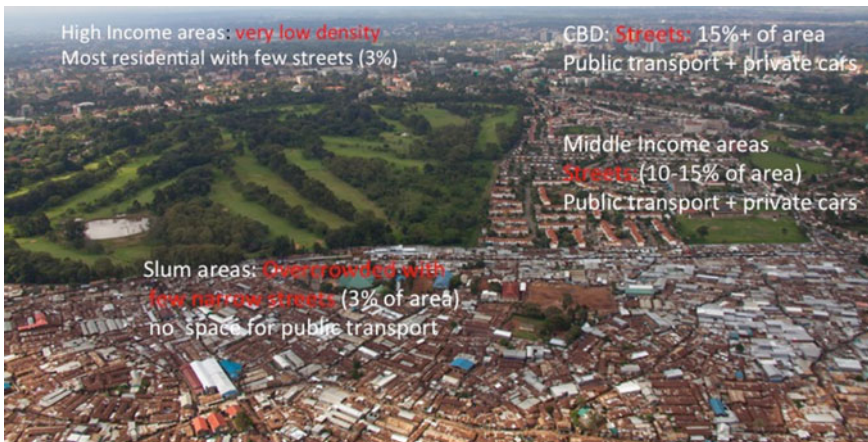
Fig. 3.16 Areal view of Nairobi with statistics on land allocated to streets in percentage. Source Mboup (2015)
