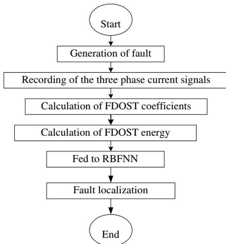
The RBFNN is trained with 12 sets of features for faults at 12 locations, and then it is tested for 7 fault locations on transmission line. The RBFNN is designed with three input vectors (features for three-phase currents) with a spread factor of 0.8. The complete flowchart is shown in Fig. 3.
