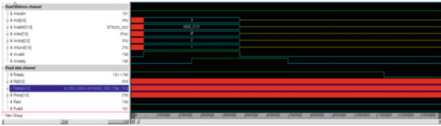
Fig. 3 Simulation result showing the read address/control signals and Arid value of 3 which is of 4 bits
