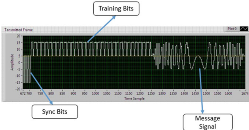
Fig. 4 Transmitted message frame
