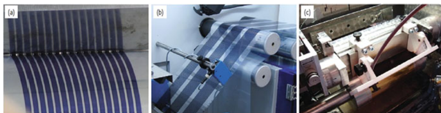
Fig. 10.2 (a) Photograph of the standing meniscus during slot-die coating of the active layer of an OSC comprising many very tightly spaced stripes. (b) A total of 48 stripes are coated simultaneously. (c) Knife coating with an open ink reservoir and a manual feed hose. (Reprinted with permission from Ref. [5])
