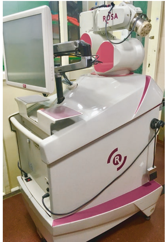
Fig. 36.1 ROSA (robotized surgical assistant) with two main parts: a computer “brain” and a robotic “arm”
