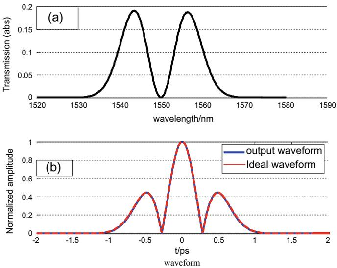
**Fig. 5** Spectrum and time domain of Gaussian pulse derived by second-order differentiators based on LPWG. **a** Spectrum; **b** time domains
