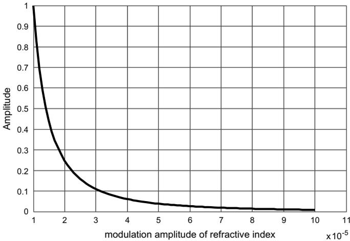
**Fig. 6** Amplitude of second-order differentiator versus  $\Delta N$
