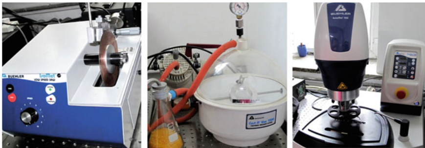
(a) Low-speed sawing slicer (b) Vacuum soaked device (c) Polishing machine
