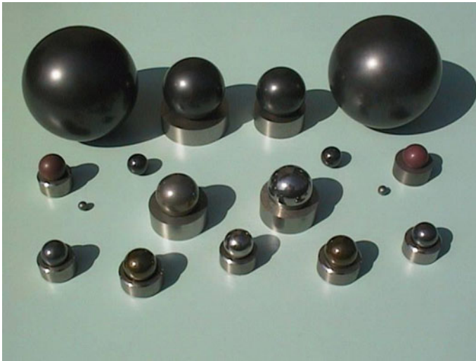
Fig. 18 Examples of finished precision ceramic balls
