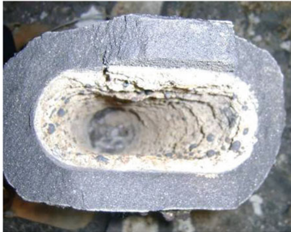
Fig. 5.3 Submerged nozzle adhered by clogs
