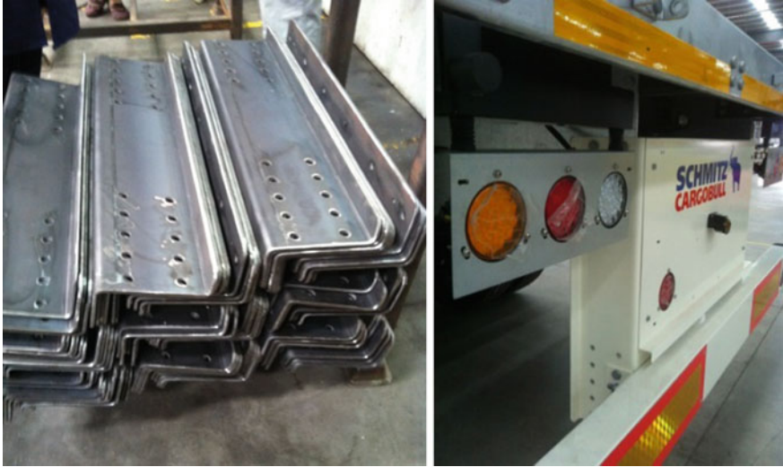
Fig. 6.33 Truck bumper beam made of S700MC
