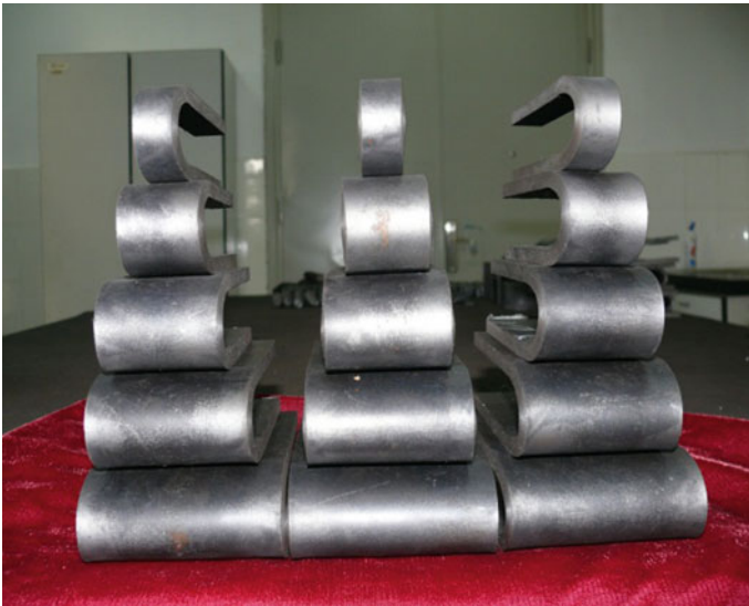
Fig. 6.76 Samples for cold bending test
