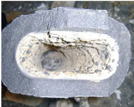
Fig. 5.3 Submerged nozzle adhered by clogs
