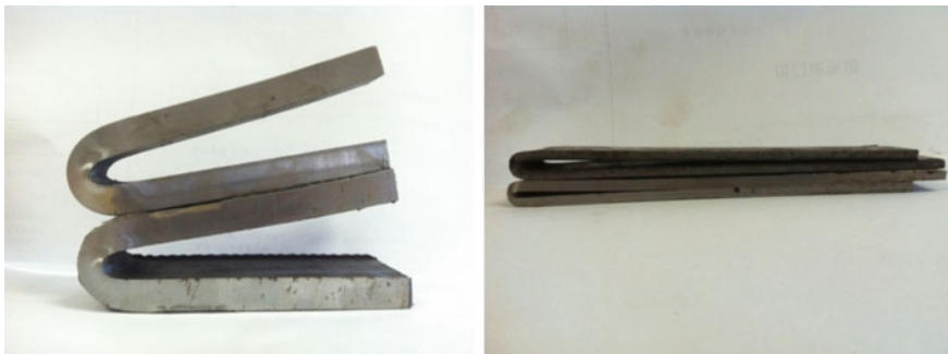
Fig. 6.25 Samples of S420MC for cold bending test
