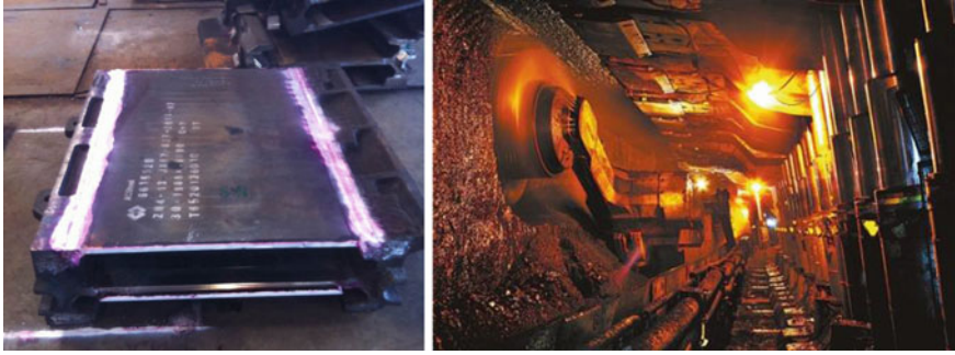
Fig. 6.57 Floors of the chute of scraper conveyor made by ZM450 plates
