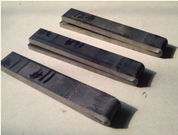
Fig. 6.41 QStE650TM samples for cold bending test
