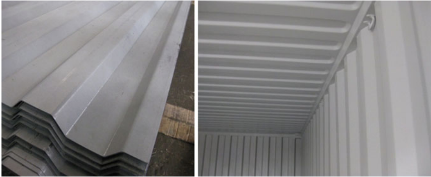
Fig. 6.16 Use of thin gauge WJX750-NH to manufacture containers
