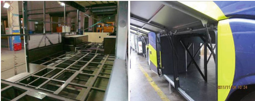
Fig. 6.34 Bus frame parts made of S700MC
