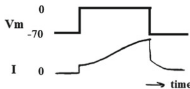
Fig. 3.12 Current in a potassium channel in response to a voltage pulse. Potassium current is positive which means that potassium ions flow outwards
