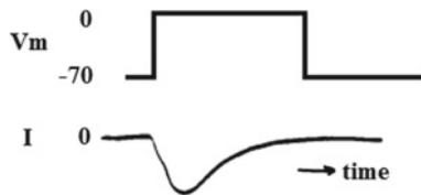
Fig. 3.11 Current in a sodium channel in response to a voltage pulse. Sodium current is negative which means that sodium ions flow inwards
