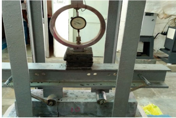
Fig. 10 Flexural strength test setup
