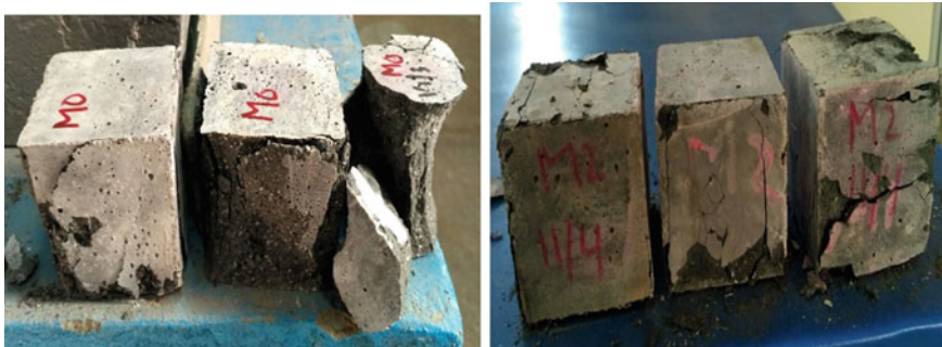
Fig. 6 Mode of failure of cube specimen with and without fiber
