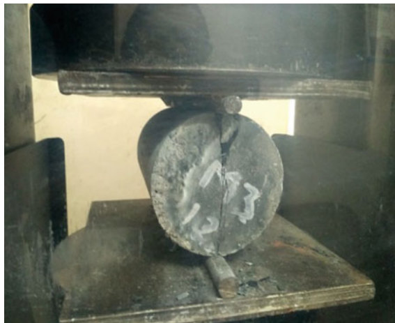
Fig. 12 Schematic picture of split tensile test setup
