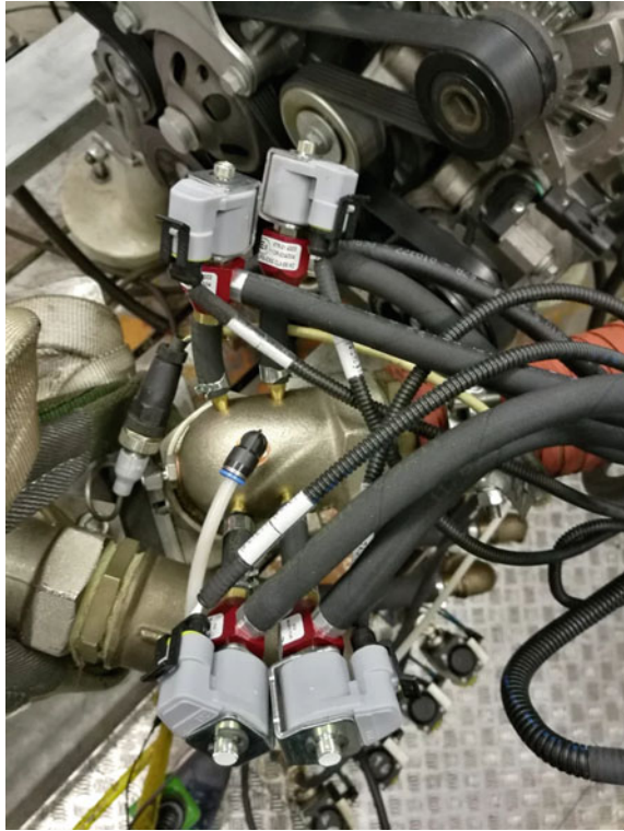
Fig. 11.16 Picture shows the installation of the four NG injectors (red and gray elements), between the intercooler and the intake manifold
