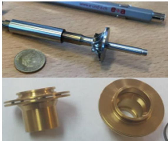
Fig. 14.23 Micro-turbine impeller and RVD as developed by MDC (Keogh et al. 2018)
