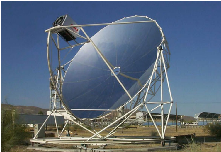
Fig. 4.8 Illustration of a parabolic disk concentrator solar cell, some specification: diameter 8.5 m, aperture 56.7 \text{ m}^2 , and average concentration factor 2500. Photo courtesy: Schlaich Bergemann and Partner
