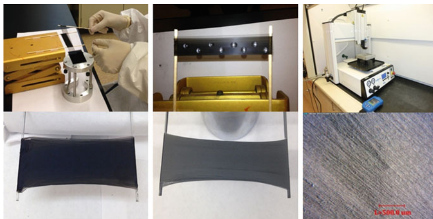
Fig. 9.6 Preparation of MWCNT sheets, and coating with NGG using robot EFD-325TT equipped with a Paasche VL-SET airbrush system
