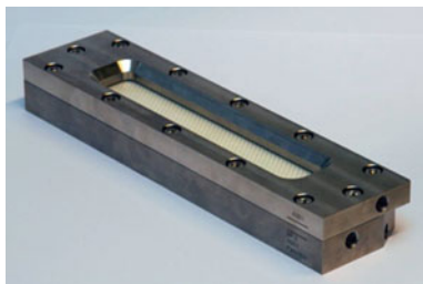
Fig. 18.5 The developed membrane fouling simulator, MFS (external dimensions of 0.07 m \times 0.30 m \times 0.04 m) with a transparent window. The MFS was operated at a pressure of 100 kPa ( \sim 14.5 psi) under crossflow and no permeation conditions (Vrouwenvelder et al. 2006)
