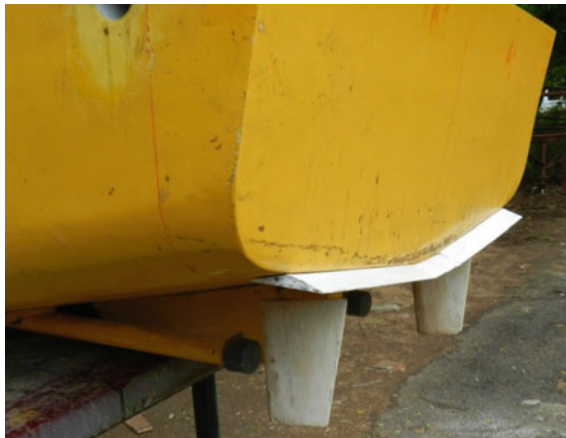
Fig. 11 Integrated wedge-flap attached to the hull
