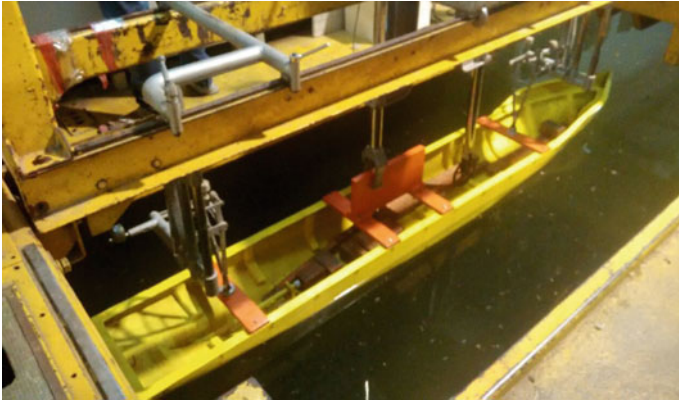
Fig. 9 KCS resistance test arrangement
