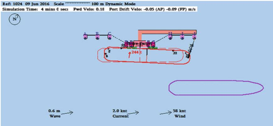
Fig. 31 Mooring arrangement with two spring lines
