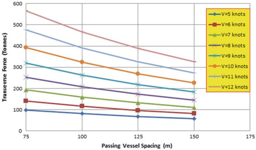
Fig. 16 Variation of transverse force with spacing of vessels
