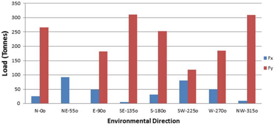
Fig. 23 Variation of environmental loads for 250,000 DWT tankers (loaded draft)
