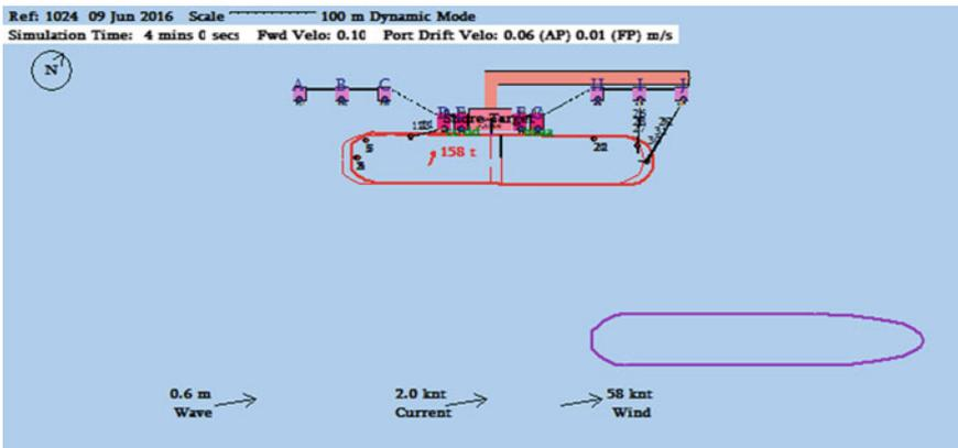
Fig. 32 Mooring arrangement with three spring lines
