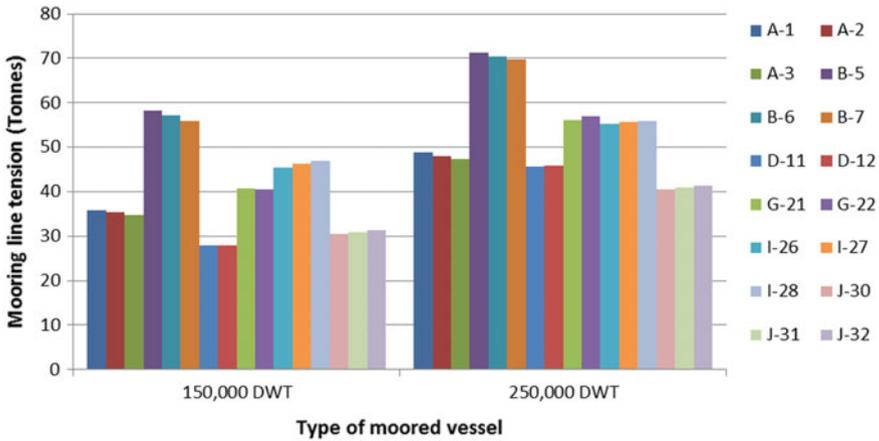
Fig. 27 Mooring line tension comparison (laden draft)
