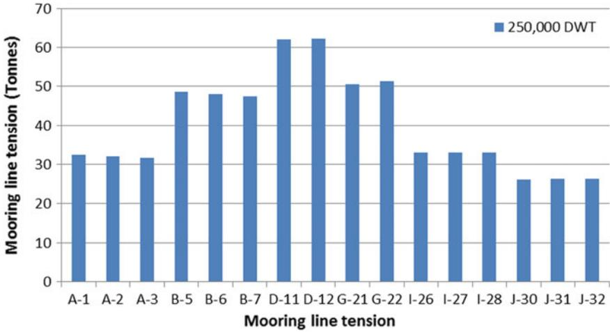
Fig. 33 Mooring line tension for 250,000 DWT
