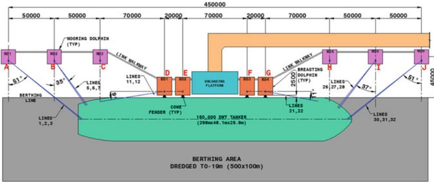
Fig. 3 Mooring layout for 150,000 DWT vessel
