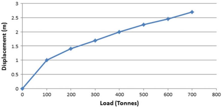
Fig. 21 Load–deflection relationship of rubber fender SCN2000 E3.0
