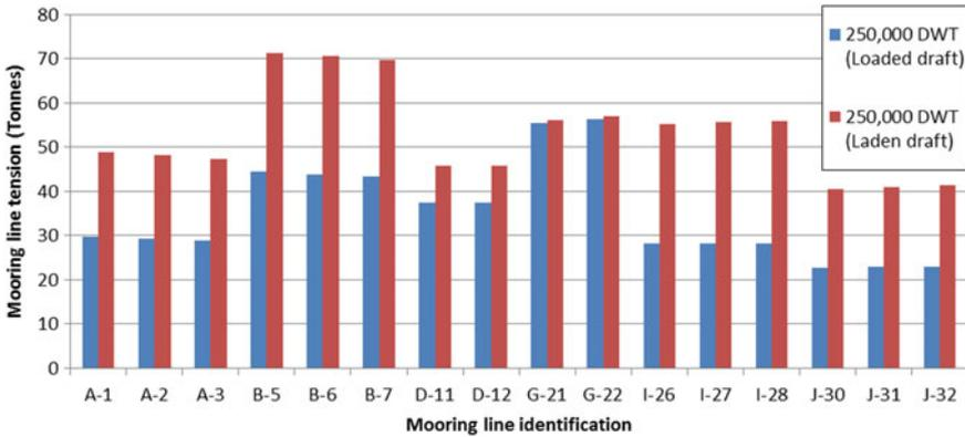
Fig. 25 Mooring line tension for 250,000 DWT
