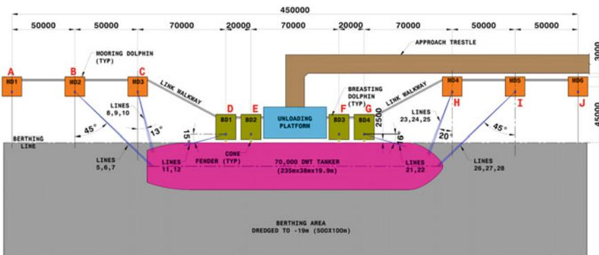
Fig. 2 Fender arrangements
