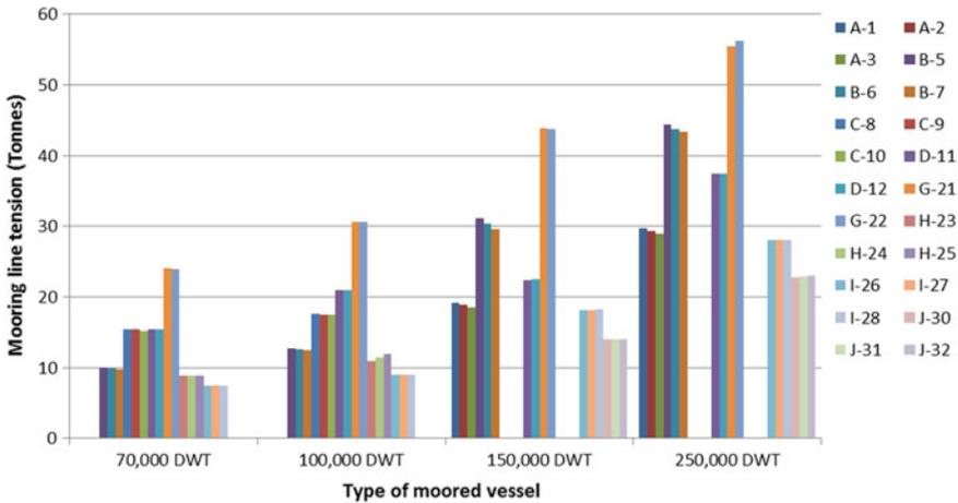
Fig. 26 Mooring line tension comparison (loaded draft)
