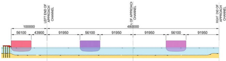
Fig. 5 Section of approach channel
