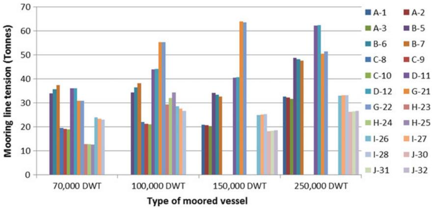
Fig. 34 Mooring line tension comparison between different moored vessels
