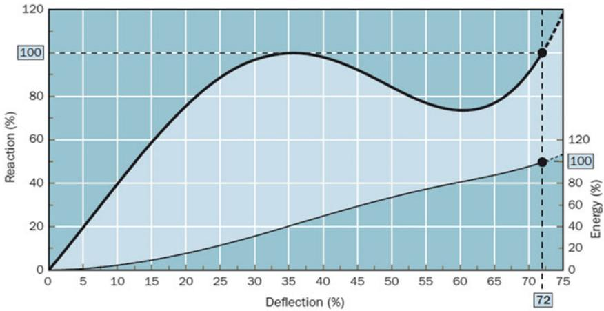
Fig. 20 Typical load–deflection relationship of rubber fender
