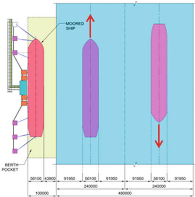
Fig. 4 Plan of approach channel
