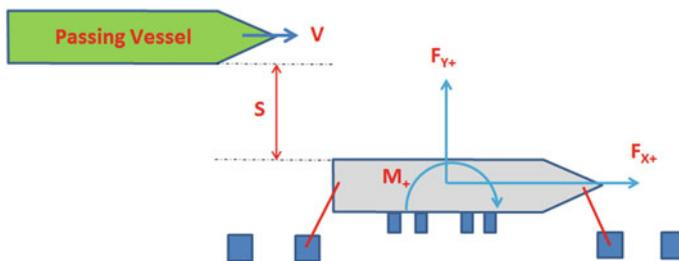
**Fig. 11** Notations used in the simulation (OPTIMOOR)
