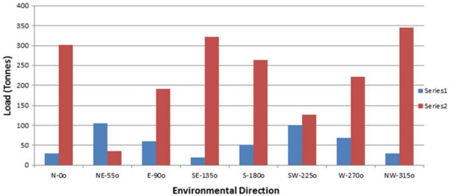
Fig. 29 Variation of passing vessel loads with environmental loads for 250,000 DWT tankers (300 m—eight knots)
