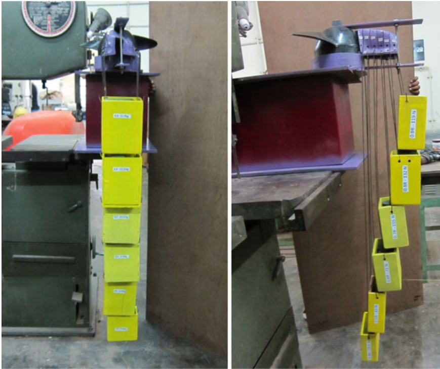
Fig. 9 A view of segment loading for static load test
