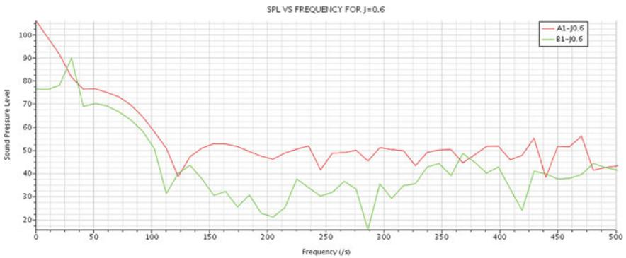
Fig. 12 SPL at receiver A1 and B1 at  $J = 0.6$
