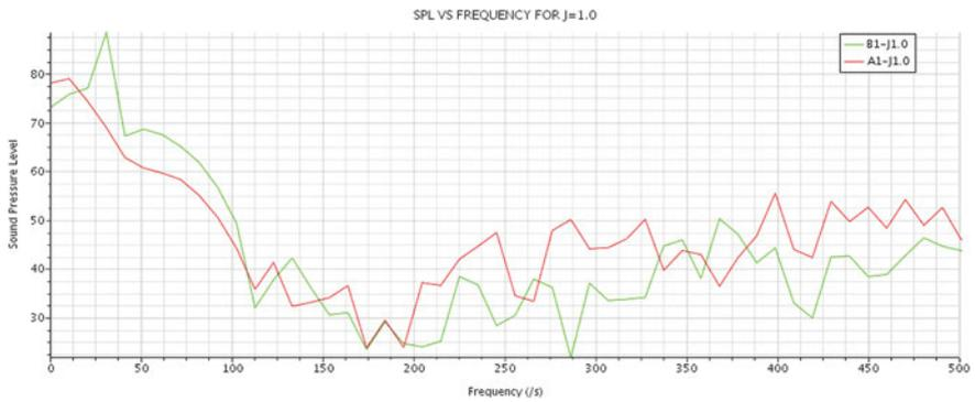
Fig. 14 SPL at receiver A1 and B1 at  $J = 1.0$
