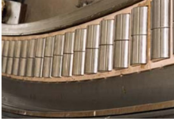
Fig. 3 Turret roller bearing with a typical diameter of 12.5 m (Courtesy of SBM) [2]
