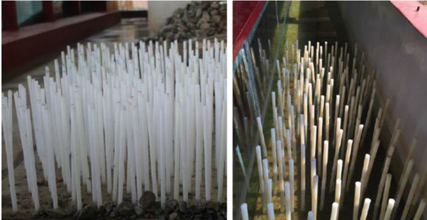
Fig. 2 Experimental model arrangement to investigate wave attenuation over emergent vegetation [1]
