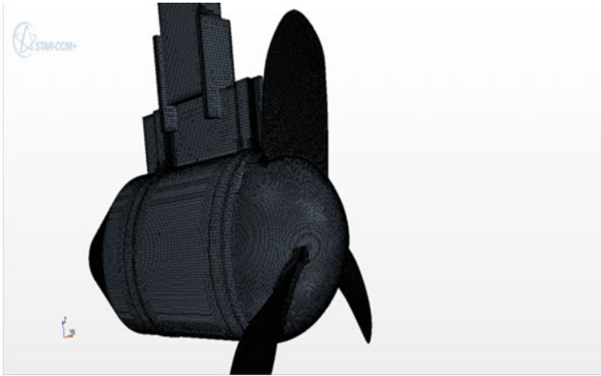
Fig. 6 A view of generated mesh for CFD studies
