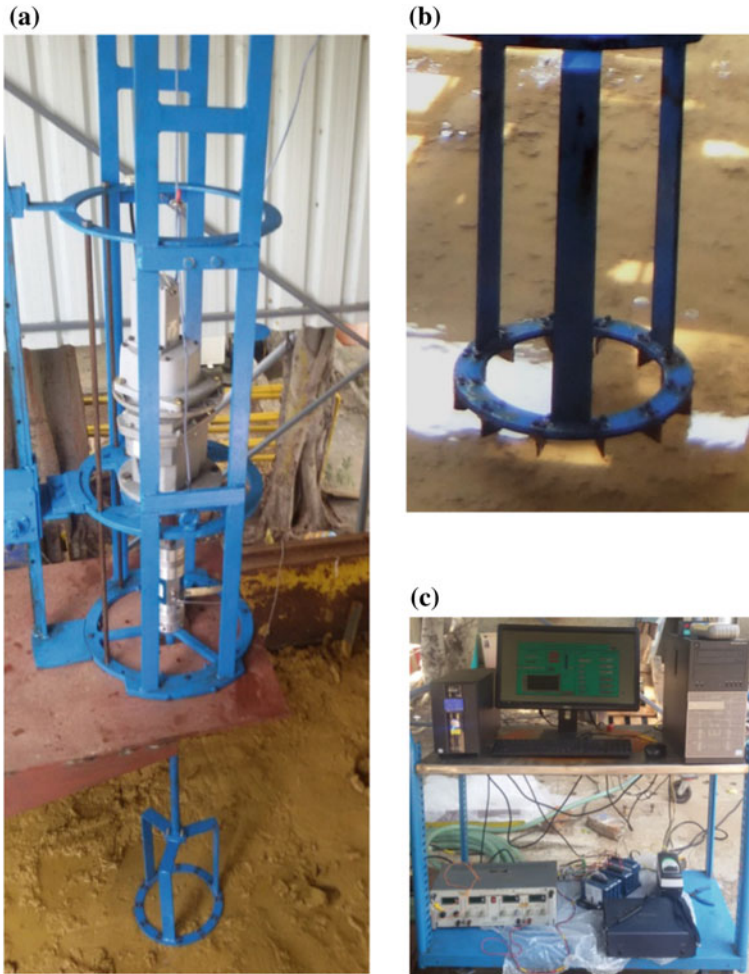
Fig. 5 Bevameter shear test setup: a bevameter shear tester, b shear ring, c data acquisition system
