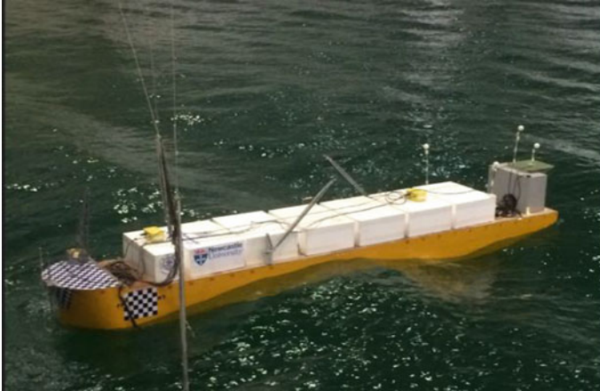
Fig. 8 Model, scale 1/64, used to represent the FPSO in deepwater Gulf of Mexico [63]
