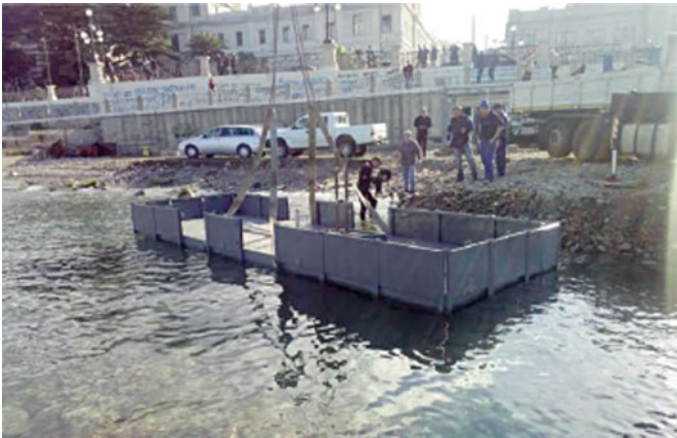
Fig. 1 Preliminary water test of the barge model at NOEL laboratory (18 vertical plates installed out of 22). Source [18]
