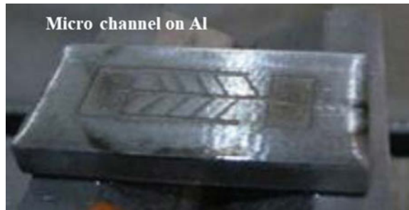
Fig. 11.32 Micro-channel heat sink on aluminum [34]
