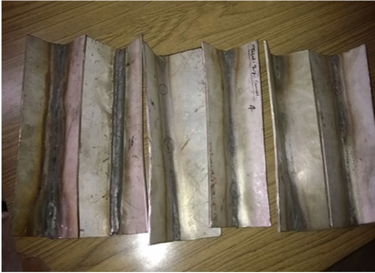
Fig. 3 AISI 304 stainless steel after bend test material
