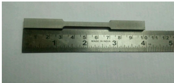
Fig. 2 Tensile test specimen with dimension
