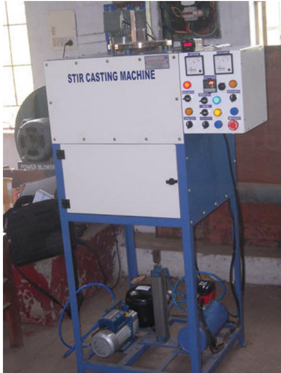
Fig. 1 Stir-casting machine set-up
