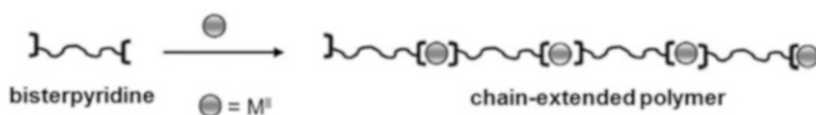
Fig. 18.27 Schematic representation of the self-assembly of bisterpyridine ligands into chain-extended polymers via metallo-supramolecular polymerization. (Figure redrawn according to [29])
