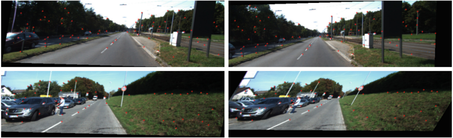
Fig. 2. The interest points extracted by RRN from the images transformed from KITTI test set with random perspective projection. Note these points are highly repeatable, which shows RRN can adapt itself to perspective projection.
