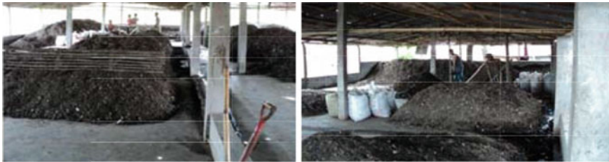
Fig. 2 Composting from Khulna City municipal solid waste by RUSTIC at Rajbandh. Source Roy et al. [6]
