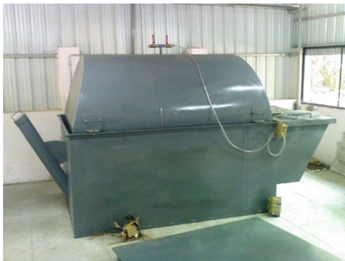
Fig. 3 The bench-scale plug flow biogas reactor (PFR) designed at CST used to convert the residue into biogas
