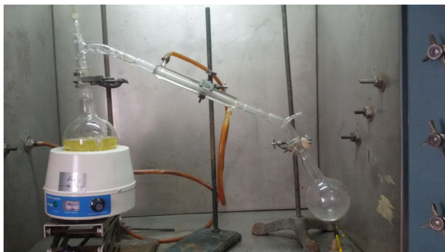
Fig. 2 Hydro-distillation process using Clevenger apparatus
