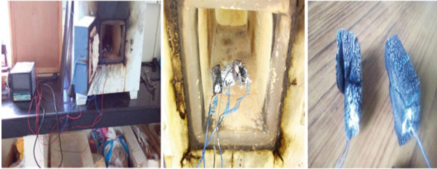
Fig. 4 Wooden pallets inside the muffle furnace
