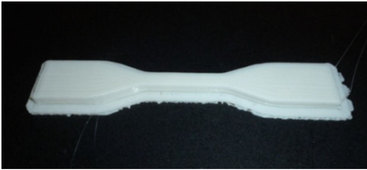
Fig. 8 3D-printed tensile specimen
