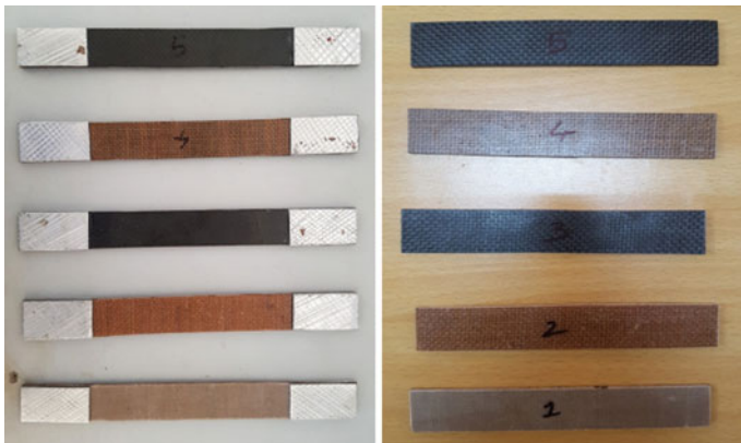
Fig. 3 Tensile and bending specimens before testing
