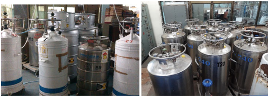
Fig. 4 Liquid helium and liquid nitrogen dewars
