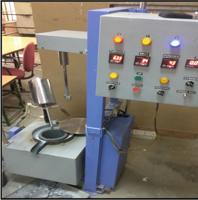
Fig. 2 Stir casting setup
