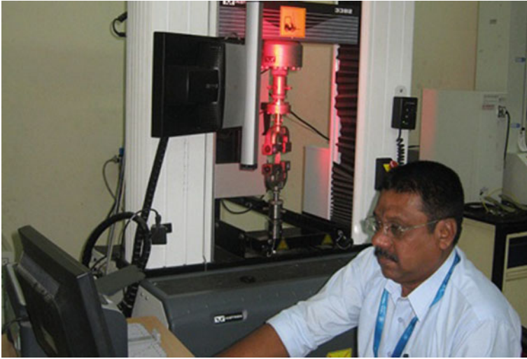
Fig. 9 Universal testing machine. Source CIPET, Hyderabad
