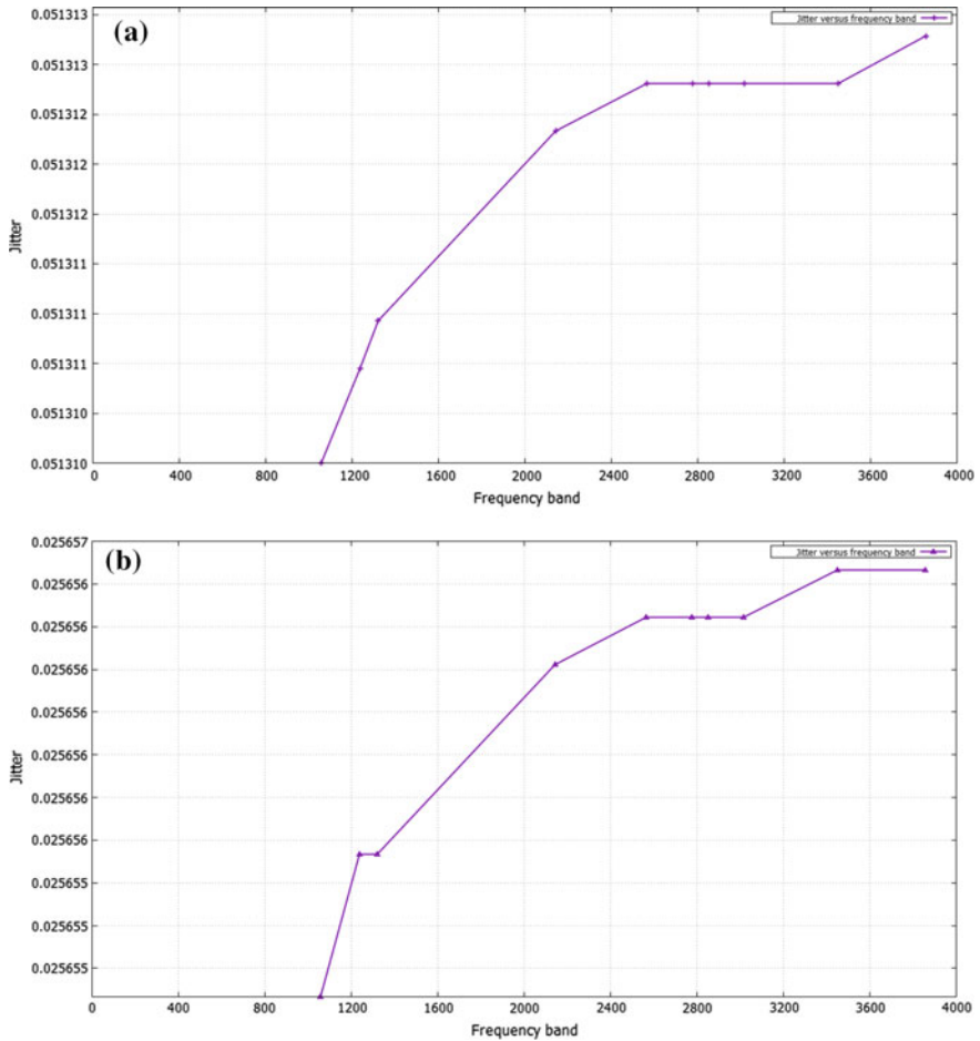
Fig. 6 a Jtr. versus operating freq. at 15 MHz channel bandwidth. b Jtr. versus operating freq. at 30 MHz channel bandwidth
