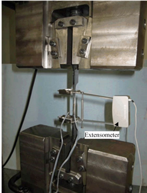
Fig. 7.8 Setup of monotonic tension coupon test of SHS columns
