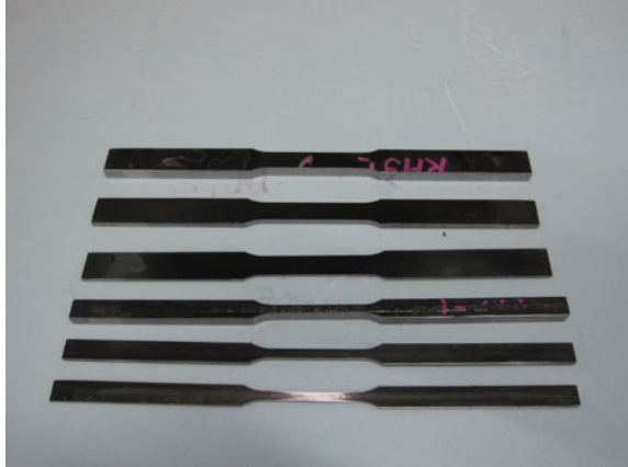
Fig. 7.6 Coupons of parallel and weld parts for SHS columns with heat treatment
