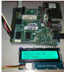
Fig. 8. “Hello world” was successfully displayed on the Grove-LCD RGB Backlight
