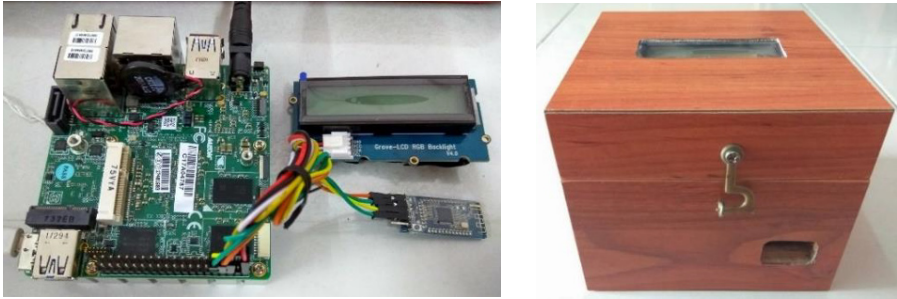
Fig. 10. The developed display device consists of UP 2 board and Grove-LCD (left), and a wooden case to store the hardware (right)
