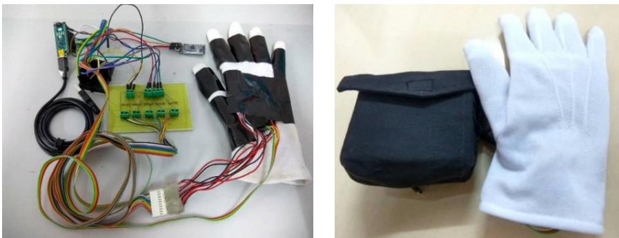
Fig. 9. The glove-based wearable. Hardware components (left), and end product (right)
