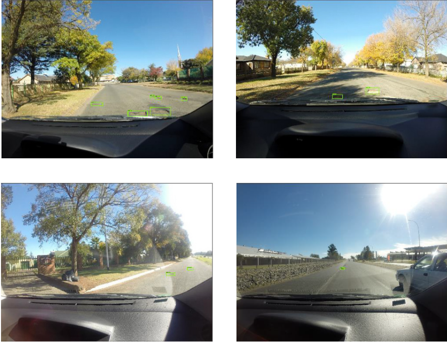
Fig. 3. Positive images with correctly identified potholes.
