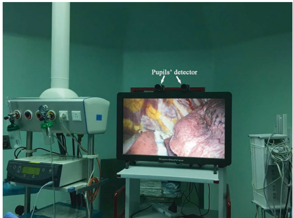
Fig. 2 The actual image of glasses-free 3D display screen with the pupils' detector
