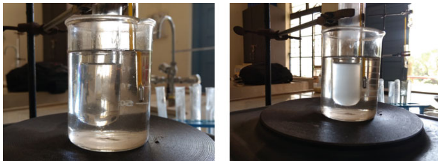
Fig. 3 Cloud point showing the effect of compatibilizer
