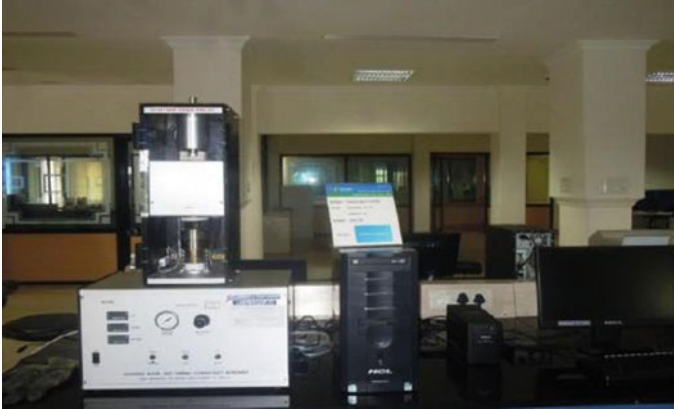
Fig. 2 Equipment used for thermal conductivity analysis Anter Unitherm Model 2022, Anter Corpo, USA available in LARPM Bhubaneswar, India.
