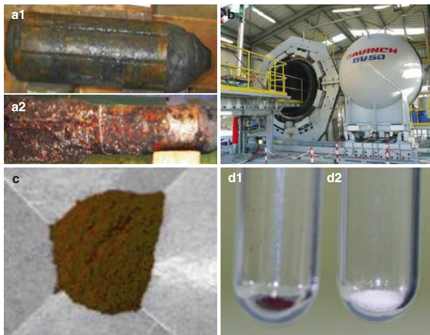
Fig. 12.2 Dismantling and detoxication of abandoned arsenical chemical weapons (containing diphenylcyanoarsine (DA) and diphenylchlorarsine (DC)) (converted to AB). The Abandoned Chemical Weapons Office operated by the Cabinet Office of Japan [24] is undertaking a project to dismantle and dispose of abandoned chemical weapons. The controlled detonation process was outsourced to Kobe Steel, Ltd. [25]. The biomimetic system was employed to convert iAs in the sample to AB [39, 40]. (a1) Abandoned chemical weapons (containing DA and DC), (a2) abandoned chemical weapons (containing lewisite + mustard gas), (b) Detonation of Ammunition in a Vacuum-Integrated Chamber (DAVINCH™), (c) fine particles produced by DAVINCH™, (d1) raw AB, (d2) purified AB
